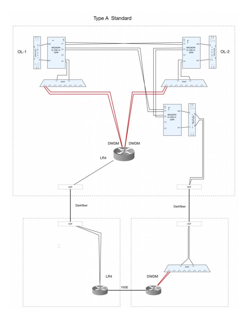
This is a more block-diagram how it will look on how it will be connected if its a Standard type of handoff. Click it for the full resolution to see how the idea is to connect things. The 8PSM "filter" is a passive splitter/combiner and is gridless.
